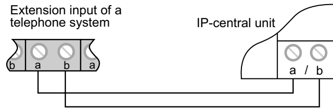
Fig. 1: Connection to the terminal strip of a PBX
