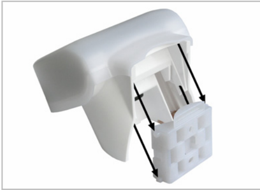
Fig. 9: Push the housing from above into the fastened mount. The bumps on the mount must snap into the rails in the housing.
