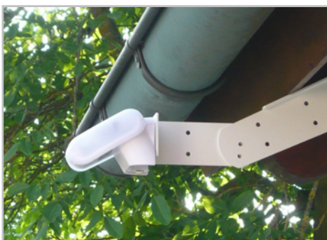
Fig. 1: The hinge arm mounting extends the weather station from under the roof eaves. Sun, wind and precipitation can thus freely act upon the sensors.
